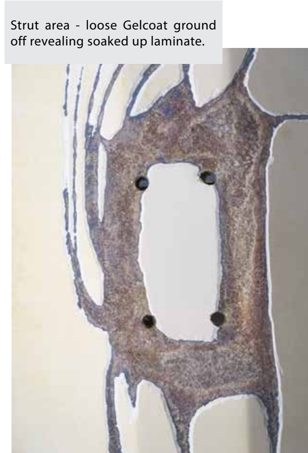
Close up. Strut area. White areas indicate bad laminate.
