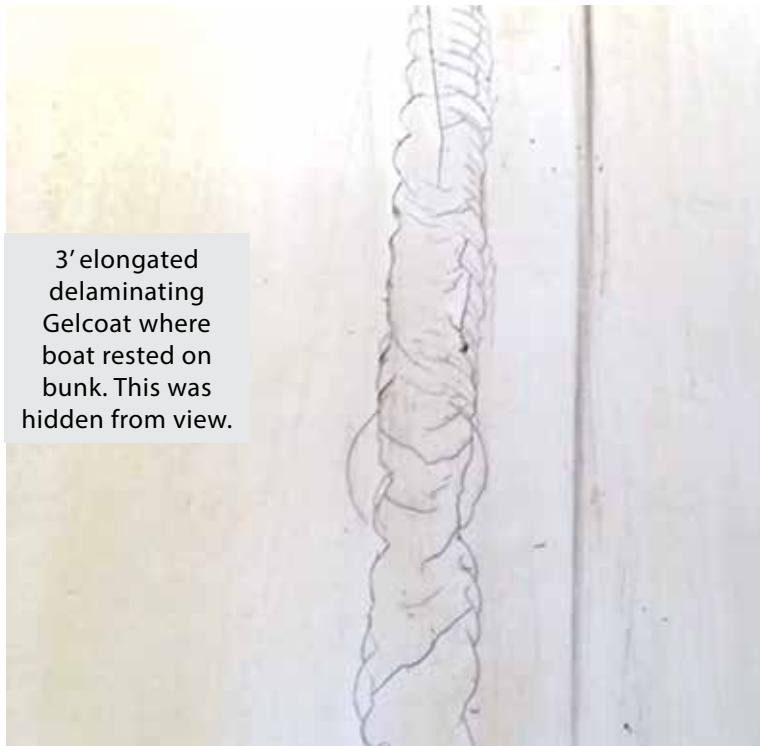
Just part of the big picture. Large areas of hull affected by water intrusion.
