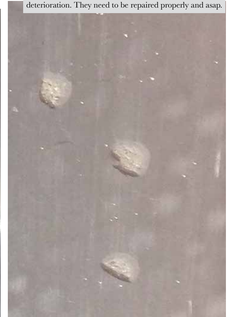
When I removed the trailer I discovered osmotic blistering on the hull in the pattern of every carpeted bunk on the trailer.
