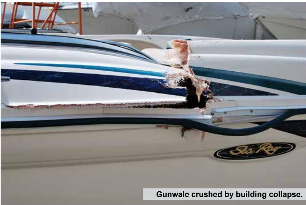
Gunwale crushed by building collapse.
