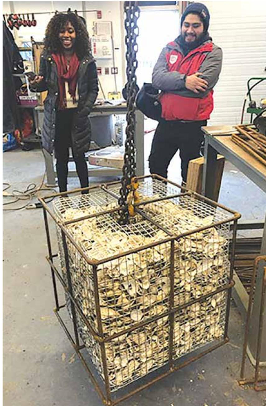
await installation into the Hudson River. Once in the Hudson, these oyster reef structures will combine to create the largest reef system in Billion Oyster Project history—covering more than 5 acres of the river. Let's take a closer look at the gabion reef structures deployed in the project and how they've evolved from conception to today.
