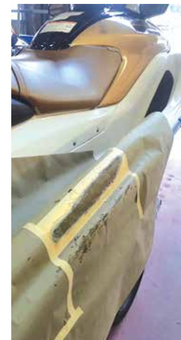
New fiberglass & resin layers applied.
