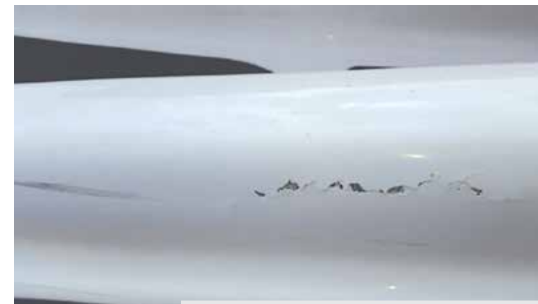
Fractured fiberglass from impact damage.
