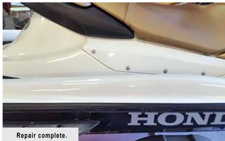
New gelcoat applied.
