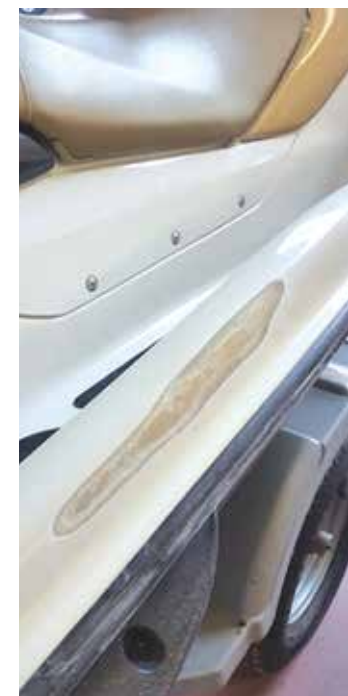
Fractured fiberglass ground off.
