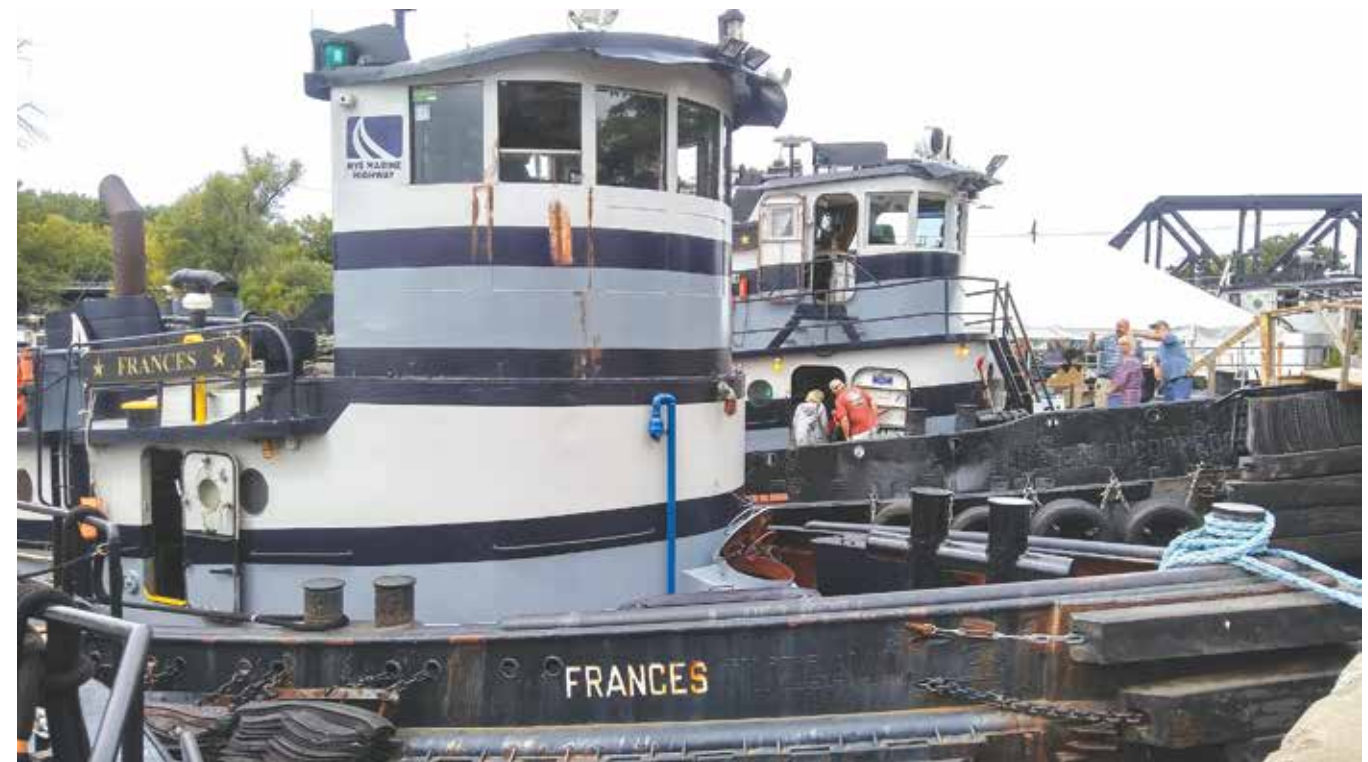
Twin sisters Margot and Frances spearhead the NYS Marine Highway Transportation Co's fleet ( www.nysmarinehighway.com ). These vessels do most of the heavy lifting on the canals these days, and were designed for such use. Their pilothouses can lower to go under those bridges made famous by the "Erie Canal Song" over a century ago.
