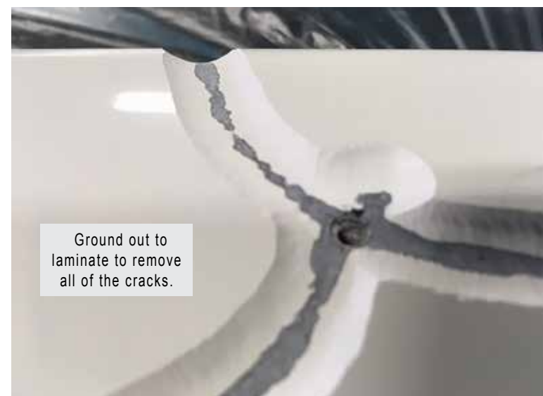
Ground cracks shows excessive gelcoat
