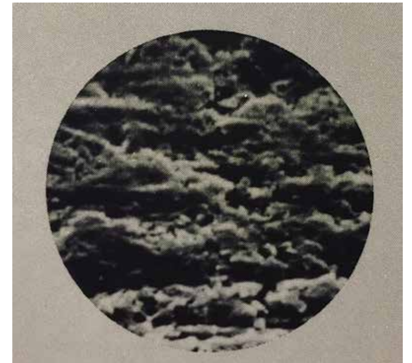
Gelcoat surface that has been sanded with 1000 grit wet sandpaper and wiped clean with a microfiber cloth
