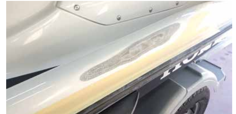
Lay up ground out, sanded and original body lines restored.
