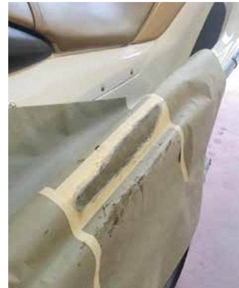
Lay up with fiberglass biaxle mat, Fiberglass cloth and resin.
