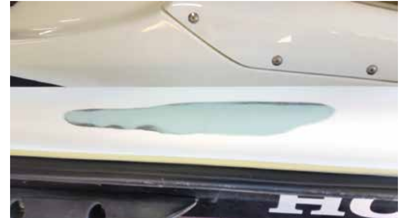
Thin layer of vinyl ester filler applied - ready for Gelcoat.
