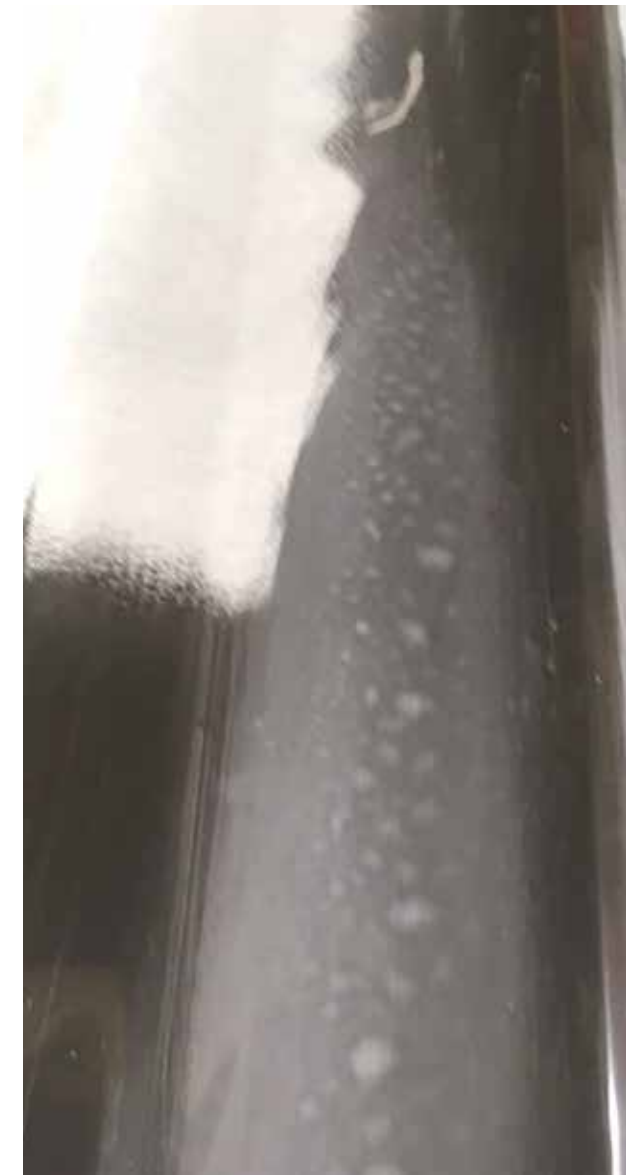
Blisters developed from resting on carpeted trailer
